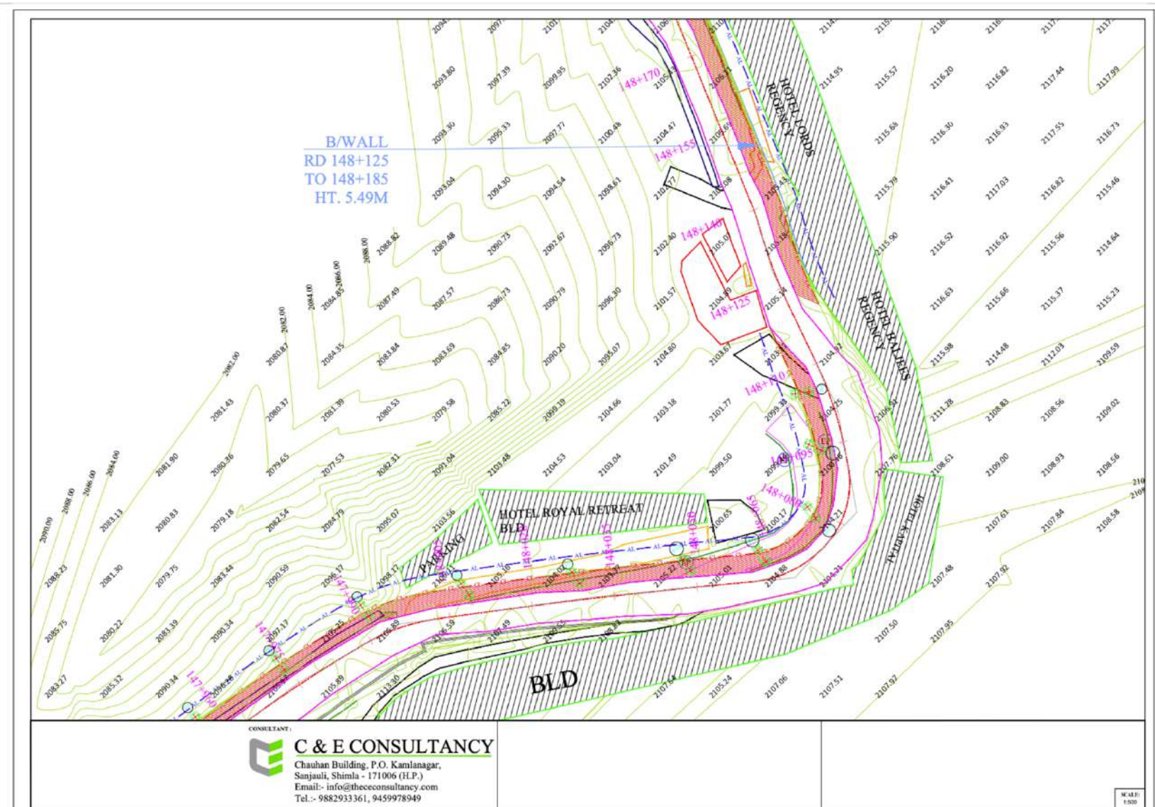
Figure 1-5: Proposed Road Design for the Improvement of MDR-67 Road Section (Victory Tunnel to Auckland Tunnel) - 2
