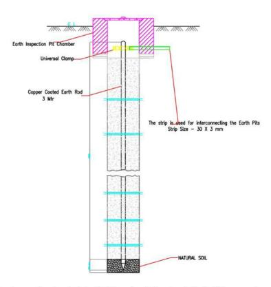
Note: we have to auger the soil up to 1mtr with 100 mm dia and fill up the pit with the 25 kg compound.
