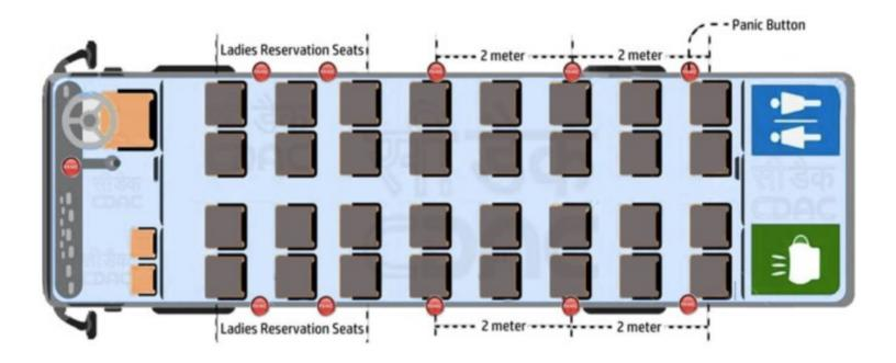
Fig: Position of panic buttons in bus
